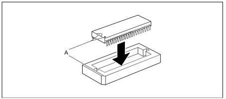
► Insert the DRAM component in such a way in the socket for video memory that the mark on the upper side of the DRAM component (A) matches the position of the mark on the socket.
